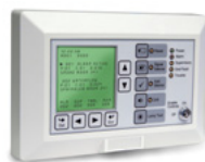
As many as eight remote annunciators mirror front panel messages and status indicators.
