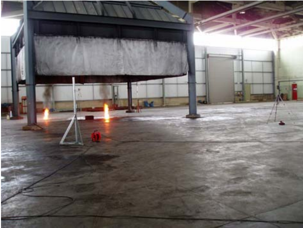
Figure 13 – Experimental configuration showing parallel camera positions
