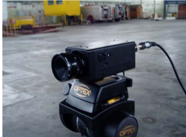
Figure 14 – Low cost B&W cameras used with the Signi-Fire system
