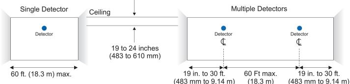
Detector positioning shown here is recommended for protected areas with flat ceilings. Spacing may vary for areas with high or sloped ceilings. In such cases, verify operation with smoke tests.
