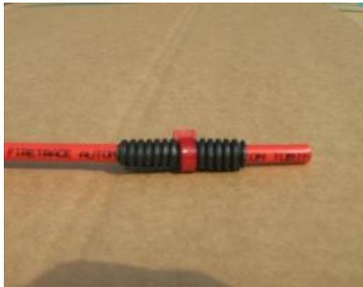
**The 8mm Detection tubing should be supported at maximum intervals of 150mm.**
