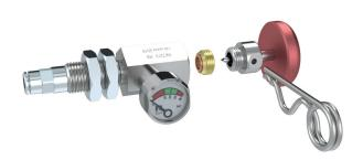
The Manual Actuator with Gauge is used when a termination of the detection line is need. It comes with a standard straight fitting that it can be changed to a tee or an elbow fitting to suit other application needs. The Pressure Indicator can be unscrewed giving access to the detection tube for pressurisation
