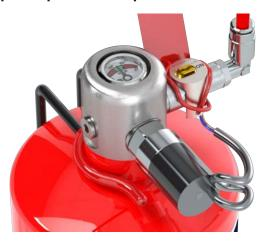
The Reacton® 1/8" BSP pressure switch is utilised where continuous monitoring of the system pressure is required, once the pressure goes past the predetermined set point the contacts will transfer and allow for a signal to be sent to your required device.
