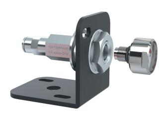
The End of Line (EOL) with Gauge is used when a termination of the detection line is required. It comes with a standard straight fitting that it be changed to a tee or an elbow fitting to suit other application needs. The Pressure Indicator is removable to allow for correct charging and maintenance. The EOL is an essential component for the system for pressure monitoring, maintenance and commissioning.
