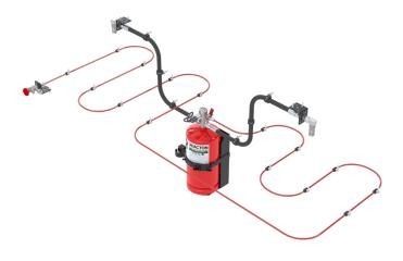
The CTX Indirect™ system utilises the Reacton® tubing as a detection only device. The tubing is installed in and around the fire risk areas. When a fire occurs, the tubing will burst at the point of highest heat.
