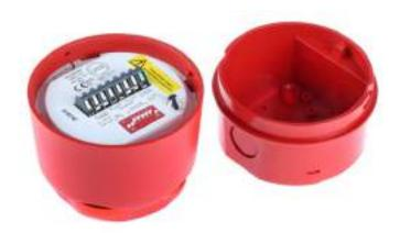
The Reacton® Sounder Beacon will be wired directly to the pressure switch from the fire suppression system. All pressure switches can be wired up either Normally Open (N/O) or Normally Closed (N/C). Depending on your installation you can utilise a 9V battery to power the unit or the power from your control panel.
